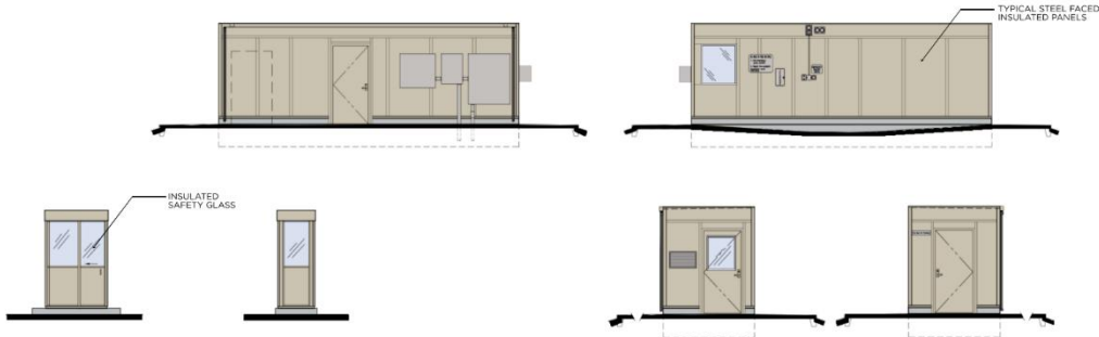
4 WARMING HUT ELEVATIONS SCALE 1:25
